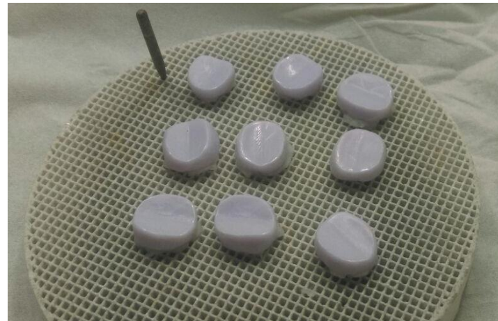
IPS e.max CAD occlusal veneers before and after crystallization
